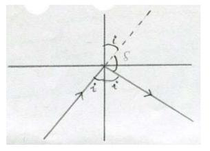
If the light incident at an angle i > c as shown in the figure the angle of deviation is given by  $\delta = \pi - 2i$
