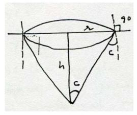
Here c: critical angle of water – air interface
