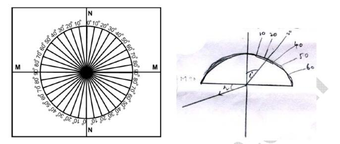
Now place a semi-circular glass disc so that its diameter coincides with the inter face line (MM) and its centre coincides with the point 'o'.
