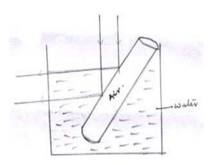
As light tries to enter air in the test tube it under goes total internal reflection bouncing back into water from the surface of the test tube giving it a shiny mirror like surface.
